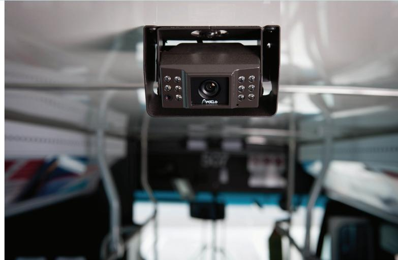
With wireless LAN capabilities, police and first responders can access live video feeds remotely from on-board cameras.
